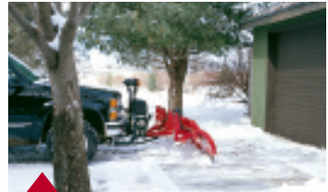
C-Plow in pull position makes backdragging driveways a breeze.
