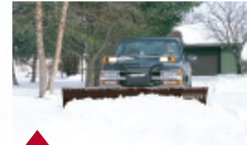
Full-featured conventional plowing with the C-Plow in push position.
